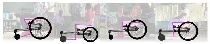
Figure 1 Wheelchair chassis of different configurations made according to the measurements and specifications collected from the clients
